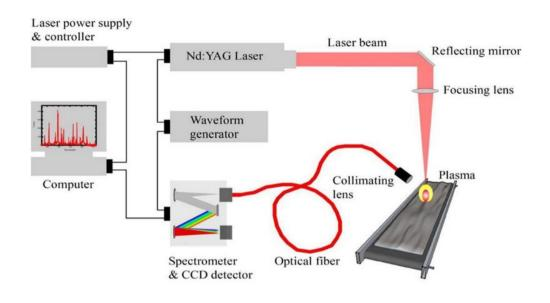
Laser-induced plasma spectroscopy(LIPS) is an elemental analysis technology developed based on the basic principle that the wavelength of atomic spectrum and ion spectrum has a one-to-one correspondence relationship with specific elements, and the spectral signal intensity has a certain quantitative relationship with the content of corresponding elements. 激光诱导等离子体光谱(LIPS),是基于原子光谱和离子光谱的波长与特定元素具有一一对应关系,光谱信号强度与相应元素的含量具有一定定量关系的基本原理而开发的元素分析技术。
